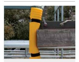
Rack Mounted Guard exceeded impact requirements of EN 15512.
